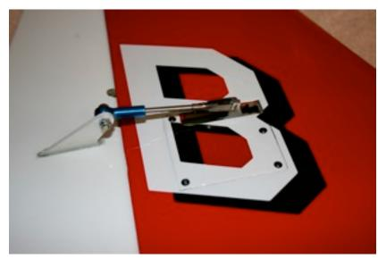
Insert rudder into aft fuse. Tighten aft locking clamp.
