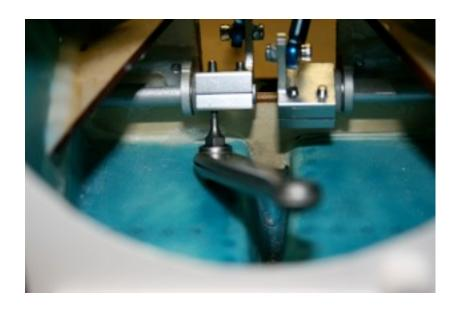
Option: For added security, chuck a #45 drill into a dremel tool and machine a small hole down through the horn block and stab spar. Insert a 1 inch 4-40 bolt or equivalent and secure with self locking nut. See photo for position of bolts.
